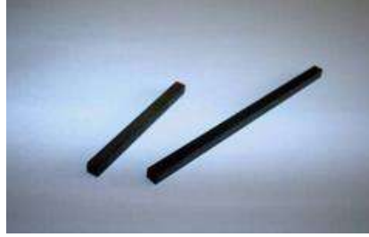
Figure 4. Shape of the electrodes, 3x3x80 mm
